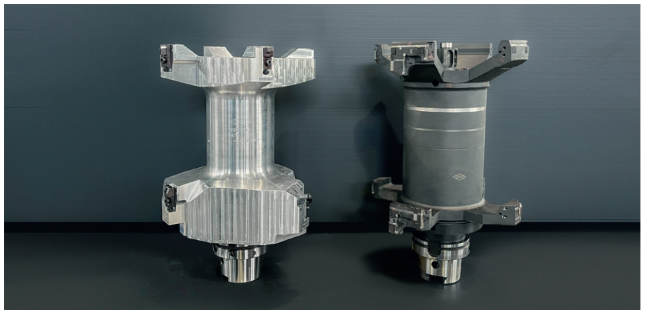
Among the 40 different tools required to produce a stator housing, two custom tools from MAPAL play a decisive role: The tool with indexable inserts for semi-finish machining (left) and a fine boring tool for finish machining.
