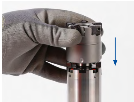
2. Clamp the milling cutter arbor in a changing device.
