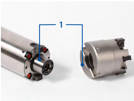
1. Clean the connection areas of the milling cutter arbor and the tool (1).
