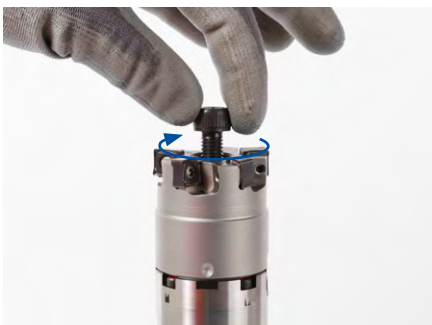
4. Lightly screw the milling cutter clamping screw into the thread bore of the milling cutter arbor by hand.
